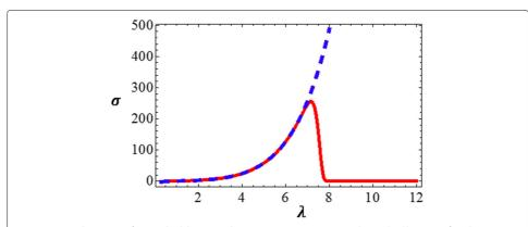
**Fig. 2** Uniaxial tension of natural rubber: Cauchy stress [MPa] versus stretch. *Dashed line* specifies the intact model; *solid line* specifies the model with energy limiter
