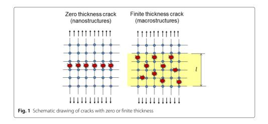
It is interesting to note that material failure does not require the breakage of all molecular or atomic bonds within a representative volume. Only fraction of these bonds should be broken for the material disintegration. For example, in the case of natural rubber, roughly speaking, every third bond should be broken within a representative volume to create a crack (Volokh 2013a).
