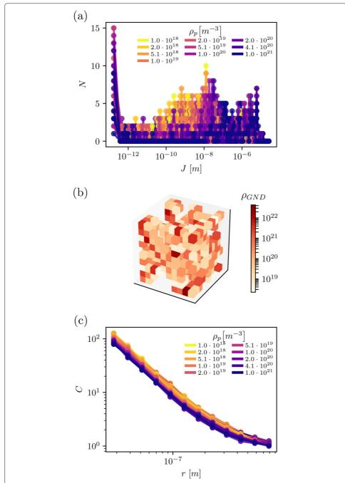
**Fig. 3** Different ways to measure the dislocation structure. **a** Distribution of dislocation junction lengthening J (Eq. 2) in single systems at  $t=2.6\cdot 10^5$  GM. The first bin also includes junctions with J=0. **b** An example of internal GND density at  $t=2.6\cdot 10^5$  GM in a system with  $\rho_p=10^{20}$  m<sup>-3</sup>. **c** Dislocation spacing correlation according to Eq. 4 in single systems at  $t=5.2\cdot 10^6$  GM
