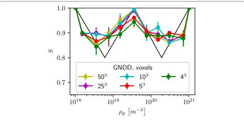
**Fig. 9** Confusion curve dependency on the number of GND density voxels. Only slight decrease of the maximum in the curve is observed depending on the number of voxels (i.e. voxel size from 280*b* to 3500*b*) when measuring GND density
