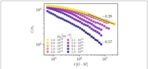
**Fig. 2** Simulations of power-law relaxation of dislocation systems with varying  $\rho_p$ . The figure shows the average strain rate during constant loading with  $\sigma_c(\rho_p)$ . The relaxation becomes more rapid and the transient time before power-law decay of  $\dot{\varepsilon}$  decreases as  $\rho_p$  is increased above some threshold value of  $\rho_p^c$
