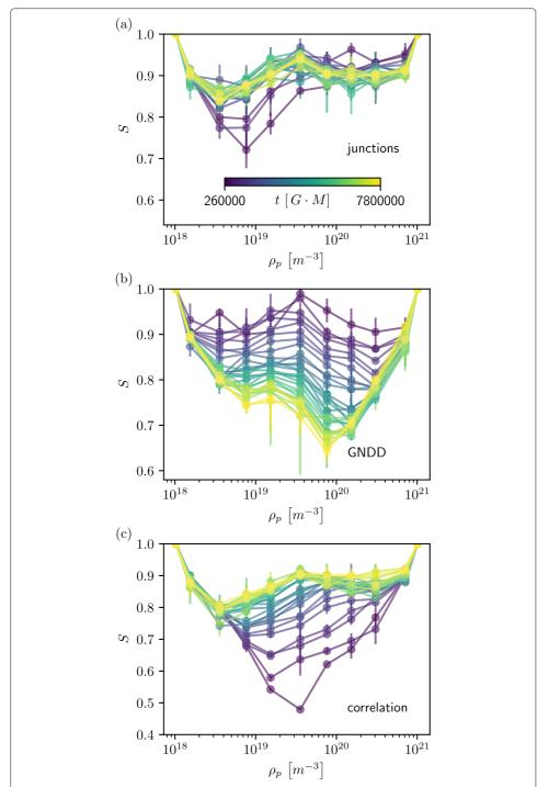
**Fig. 7** The confusion curves with two principal components of single time step snapshot. Used features are **a** junction lengthening, **b** GND density change, **c** dislocation correlation. The number of collected systems starts to decrease after  $t = 4.7 \cdot 10^6$  GM
