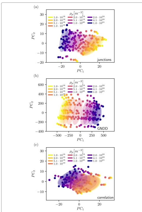
**Fig. 4** The systems represented by the two first principal components. The descriptors are **a** junction lengthening **b** GND density change and **c** dislocation correlation collected during the simulation time interval. The coloured regions come from a fit of bivariate normal distribution on the data sets of different  $\rho_p$  to visualize the differences between them
