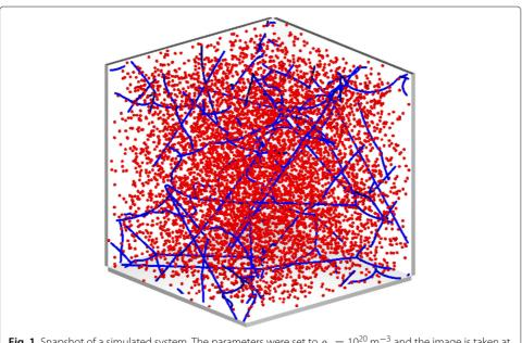
**Fig. 1** Snapshot of a simulated system. The parameters were set to  $\rho_p=10^{20}~\rm m^{-3}$  and the image is taken at  $t=10^{-9}~\rm s=2.6\cdot 10^5$  GM, where  $M=M_{\rm edge}=M_{\rm screw}$
