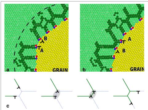
**Fig. 6** Effective climb (see text). Direct interaction of two dislocations A and B with Burgers vectors [100] and  $1/2[1\sqrt{3}0]$ : **a** initial configuration; **b** final configuration; **c** sketch of the mechanism. The dashed line indicates the initial position of the grain boundary. The color code is the same as the one used in Fig. 5
