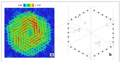
**Fig. 9 a** Color map of the residual atomic displacement magnitude after the grain disappeared ( $\theta = 10^{\circ}$ ); **b** simplified description of the grain boundary used to develop the toy model of grain boundary migration
