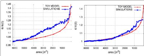
**Fig. 11** Evolution of the misorientation  $\theta$  as a function of the grain size predicted by the toy model (in red) compared with the results obtained by atomistic simulations (in blue) for  $\theta_0=10^\circ$  (left) and for  $\theta_0=15^\circ$  (right)
