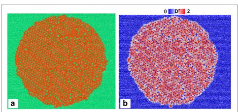
**Fig. 14** Atomic structure after the grain shrinkage ( $\theta_0 = 21.8^\circ$ ): **a** atoms that have not changed their first nearest neighbors shell are represented in green; **b** atoms are colored according to the value of the  $D^{(n)^2}$  coefficient (see text for details)
