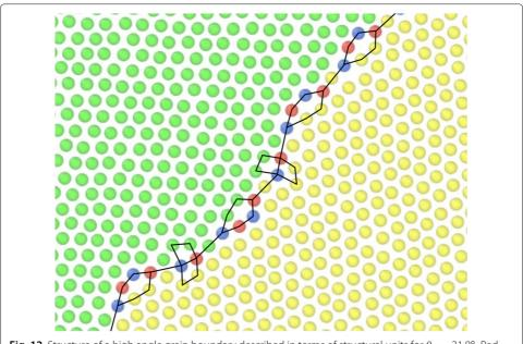
**Fig. 12** Structure of a high angle grain boundary described in terms of structural units for  $\theta_0=21.8^\circ$ . Red and blue atoms have 5 and 7 NN, respectively
