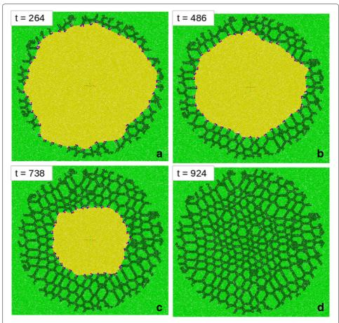
**Fig. 8** History of the 5-7 defect pair during the grain shrinkage (dark green) at reduced time **a**) t = 264, **b**) t = 486, **c**) t = 738, **d**) t = 924. Their traces form a regular pattern of hexagonal-shaped cells (for the color code see Fig. 5)
