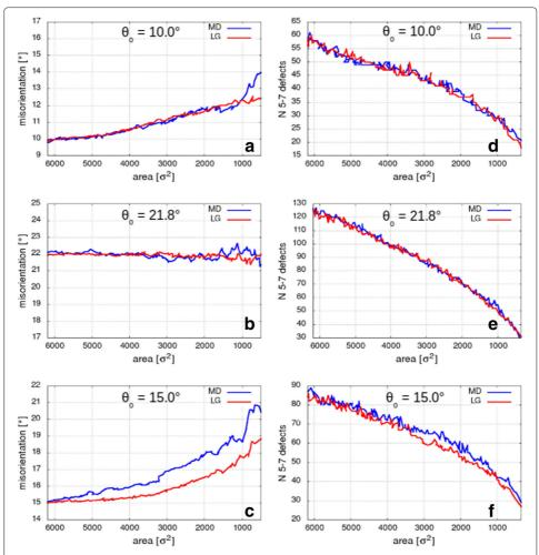
**Fig. 2 a-c** Evolution of the misorientation angle  $\theta$  and (**d-f**) of the number of 5-7 defects along the grain boundary as a function of the grain area, for the initial values  $\theta_0 = 10^\circ, 21.8^\circ, 15^\circ$ . The results obtained with the LD model (red) are compared with the ones obtained with MD simulations (blue)
