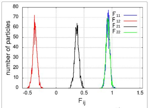
**Fig. 15** Histogram of the deformation gradients inside the grain for atoms such that  $D^{(n)^2} < 0.1$  after the grain shrinkage ( $\theta_0 = 21.8^{\circ}$ )
