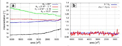
**Fig. 13 a** Misorientation as a function of the grain area (in  $\sigma^2$  units) for several initial misorientation  $\theta_0$ ; **b** 5-7 pairs density  $\rho_{5-7}/\rho_{5-7_0}$  along the grain boundary (red curve) and change in the misorientation angle  $\theta/\theta_0$  (blue curve) during grain shrinkage for the initial misorientations  $\theta_0 = 21.8^{\circ}$
