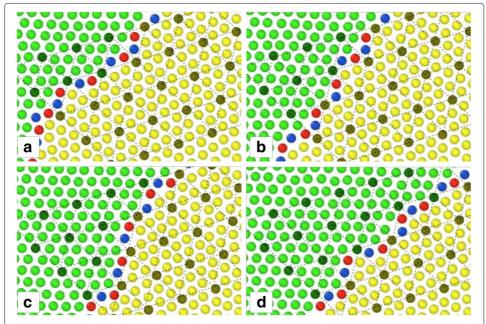
**Fig. 16 a-d** 5-7 defects walk during grain shrinkage for  $\theta_0=21.8^{\circ}$ . Atoms on the  $\Sigma$ 7 coincidence site lattice are shown in black, the coincidence sites grid in dotted line
