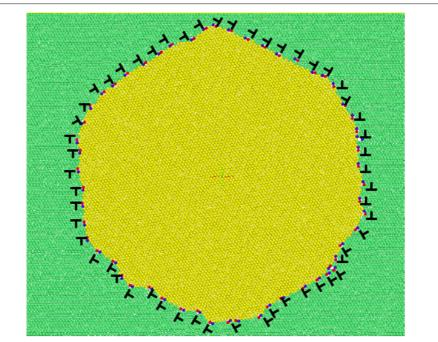
**Fig. 3** Facet formation during grain shrinkage for an initial misorentation  $\theta=10^\circ$ . The matrix is represented in green and the grain in yellow. Each dislocation is shown by a 5-7 pair (blue-red). Each facet is composed of a set of dislocations having the same Burgers vector
