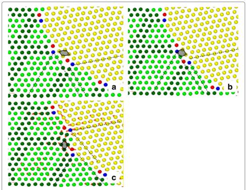
**Fig. 7** Effective climb (see text): **a** two dislocations approach each other (center of the figure); **b** they arrive at a distance comparable to two interatomic spacings, thus inducing a strong distortion in the surrounding lattice; **c** a local slip of atoms induces a rotation of the original Burgers vector (atomic displacements are represented by arrows). For the color code, see Fig. 5
