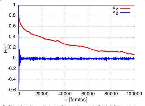
**Fig. 1** Normalized auto-correlation function of the second component of the velocity (blue curves) and position (red curves) of an atom obtained in MD at  $T=0.125\epsilon_{LJ}/k_B$
