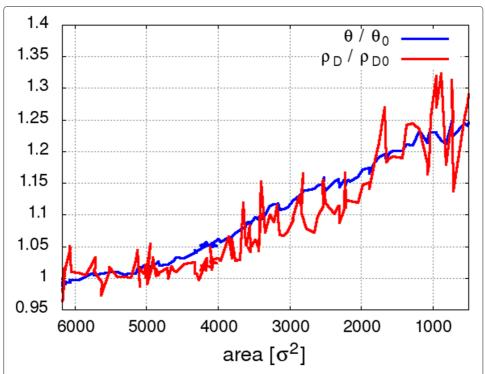
**Fig. 4** Evaluation of the dislocation density  $\rho_D/\rho_{D_0}$  along the grain boundary (red curve) and change in the misorientation angle  $\theta/\theta_0$  (blue curve) during grain shrinkage for  $\theta_0=10^\circ$
